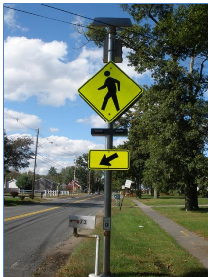
Rapid Rectangular Flashing Beacon (Pedestrian Warning Sign, pedestrian actuated)
