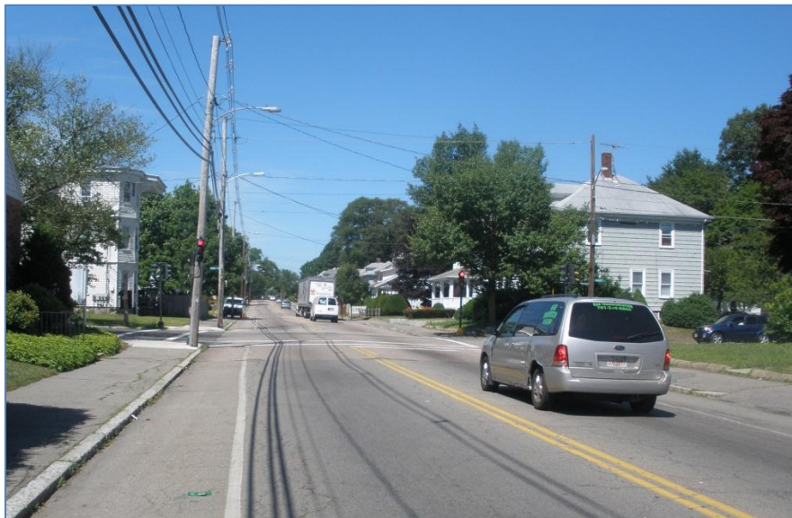
Intersection of Forest Avenue/Manomet Street/Bouve Avenue showing pole mounted signals, the signal head on the left is mounted on a utility pole, the picture is from Forest Avenue looking westbound
