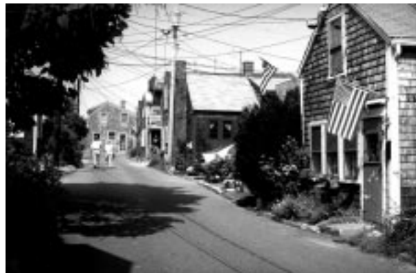
Streets in village centers may not need sidewalks if traffic is slow and infrequent and sidewalks would impact the village character. (Bearskin Neck, Rockport)
