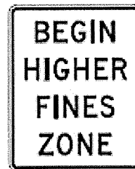
Figure 3 – Higher Fines Zone, as supplement to placard to school zone signs, and when legislation allows
