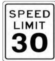
Typical Speed Limit Sign (R2-1)
