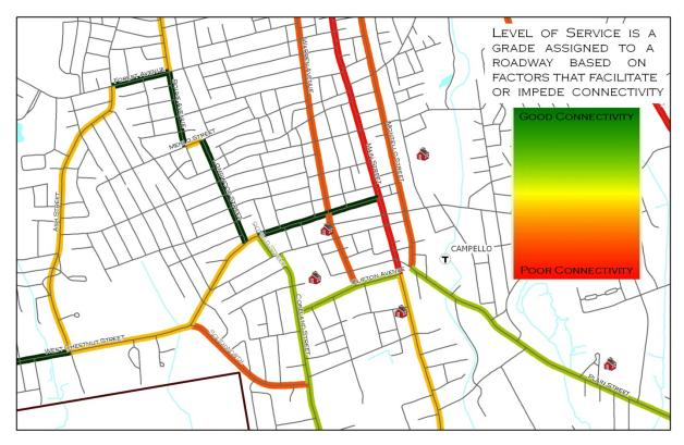
Figure 9: Example of Bicycle and Pedestrian Level of Service Findings
