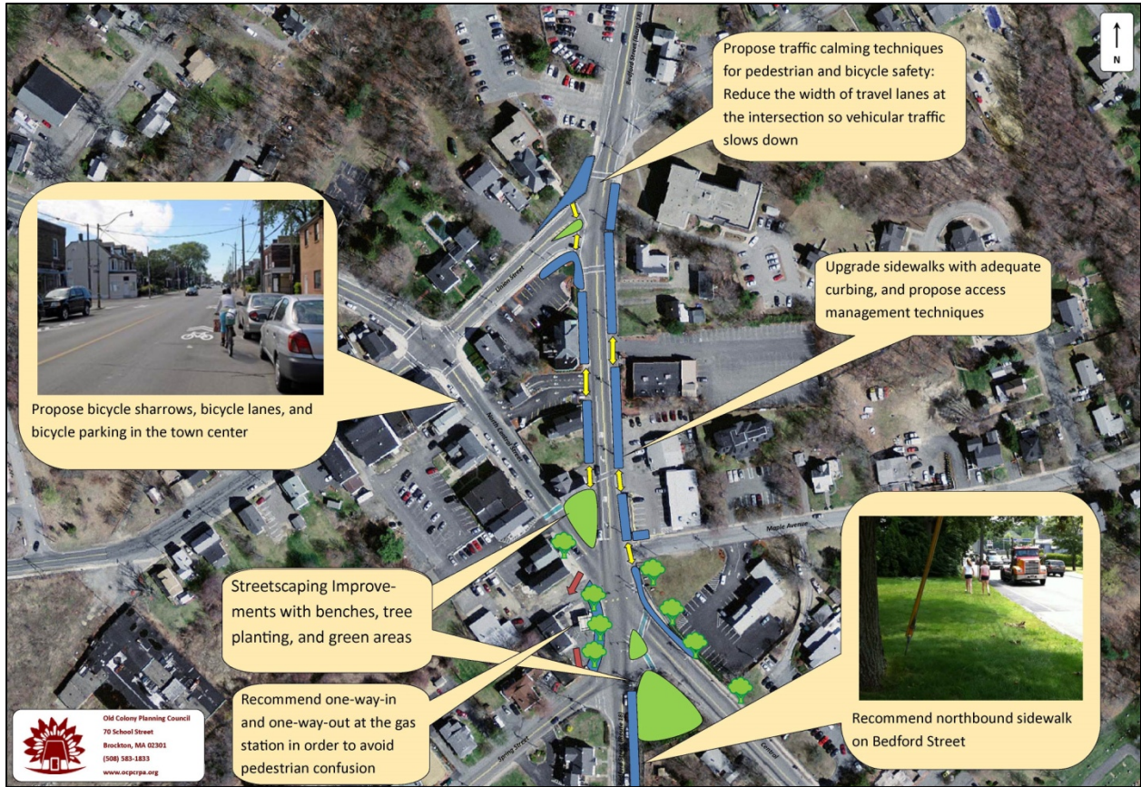
Figure 10 Potential Pedestrian/Bicycle Improvements to East Bridgewater Center
