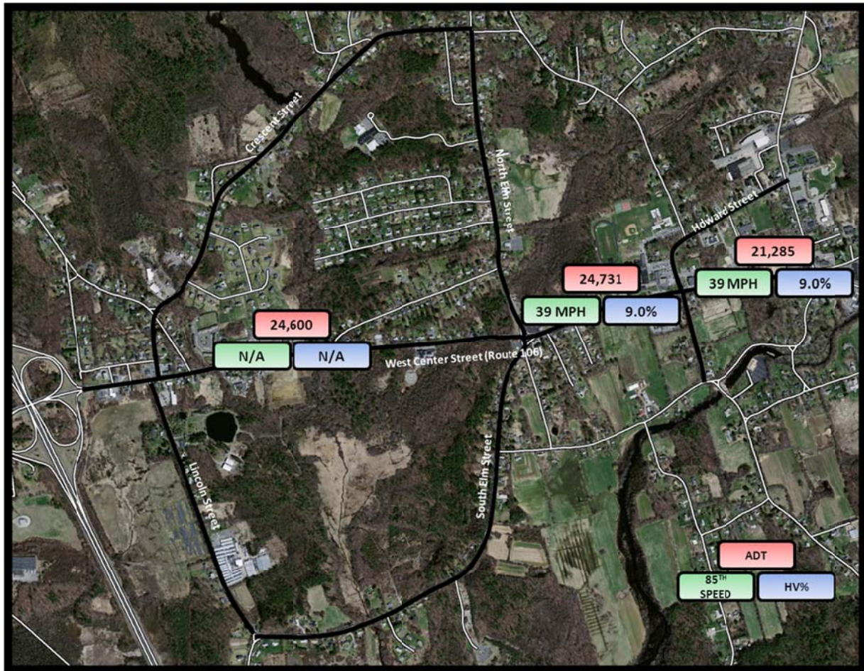
Figure 3 West Bridgewater Average Daily Traffic (ADT), 85 th Percentile Speeds, and Percent Heavy Vehicles
