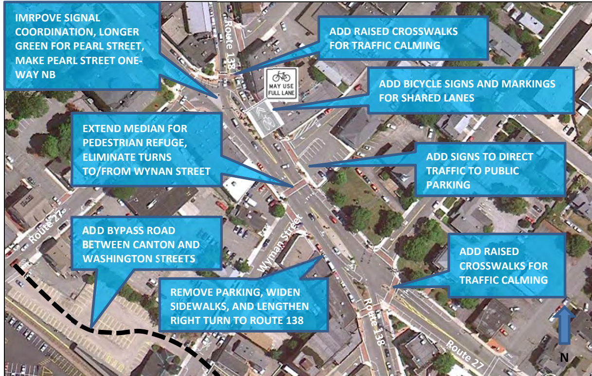
Figure 22 – Improvements to Stoughton Center
