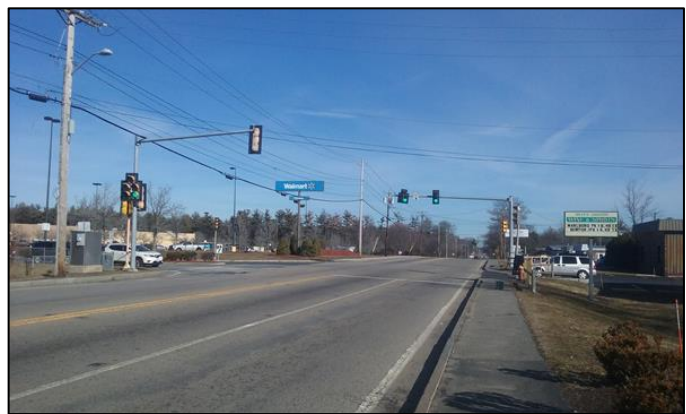
Figure 17 - Although Route 123 has a sidewalk on the south side, there are no crosswalks and no pedestrian signals and actuation at the Wal-Mart/Route 123 intersection in Abington.
