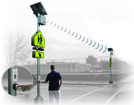
Pedestrian Actuated Rapid Rectangular Flashing Beacon
