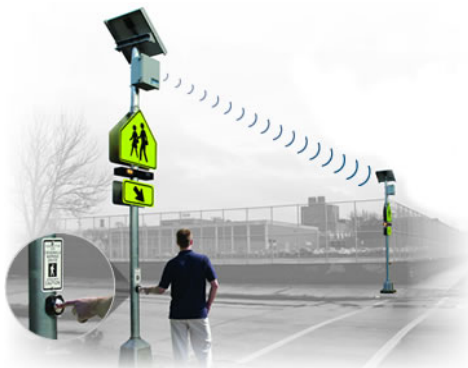
Pedestrian Actuated Rapid Rectangular Flashing Beacon
