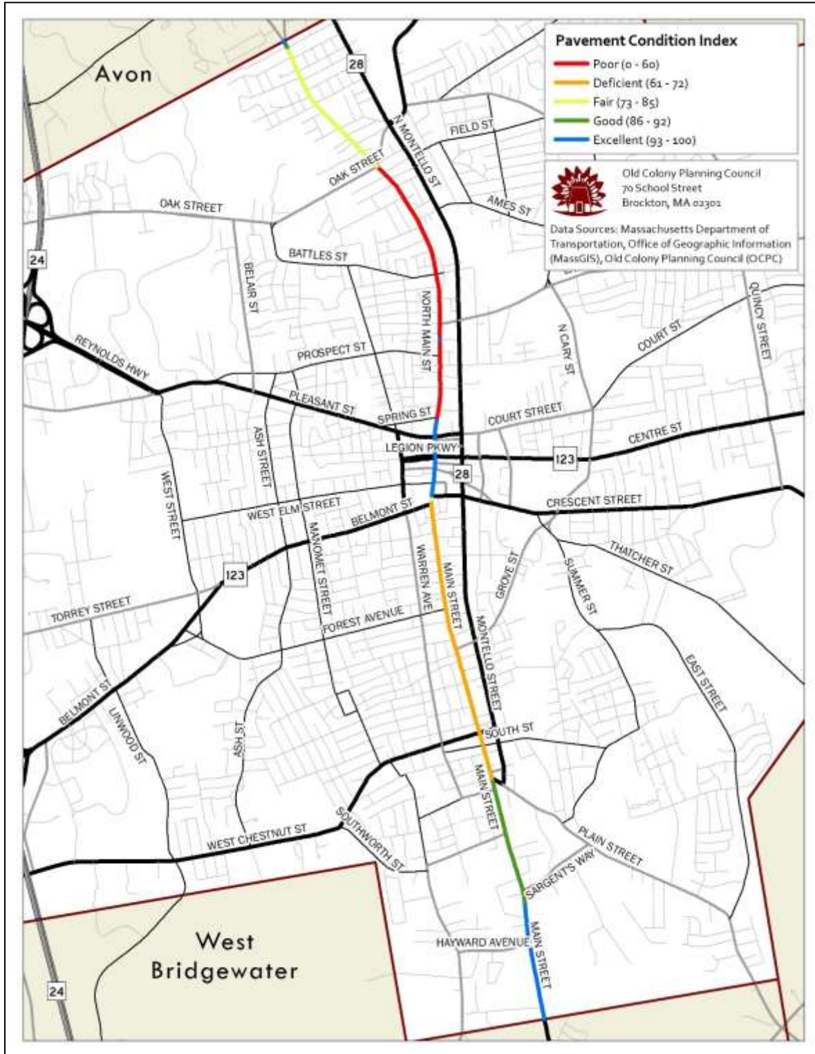
Figure 16 – Main Street Brockton Pavement Conditions
