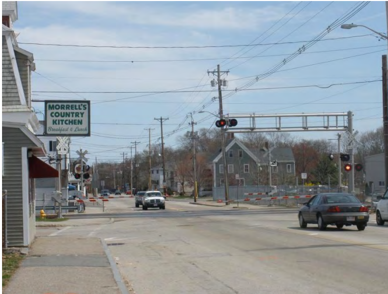
Photo: Crossing gates in down position at North Avenue MBTA crossing.
