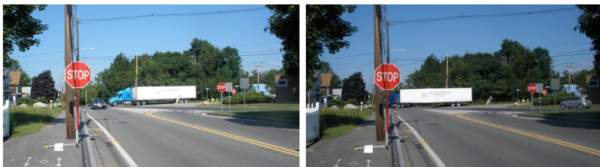
A tractor-trailer truck exiting Tosca Drive headed west on Central Street (Route 27) encroaches on the Central Street (Route 27) eastbound travel lane
