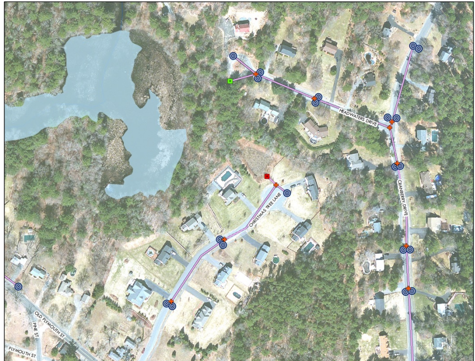
Figure 5. Detail of catch basins, pipes, junctions, and outfalls near Christmas Tree Lane in Halifax.
