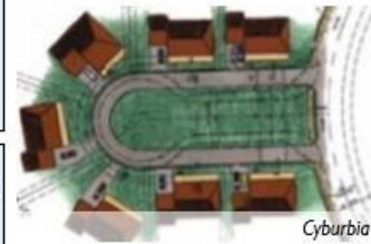
An alternative cul-de-sac design that allows for recreational space as well as a place to improve stormwater infiltration.
