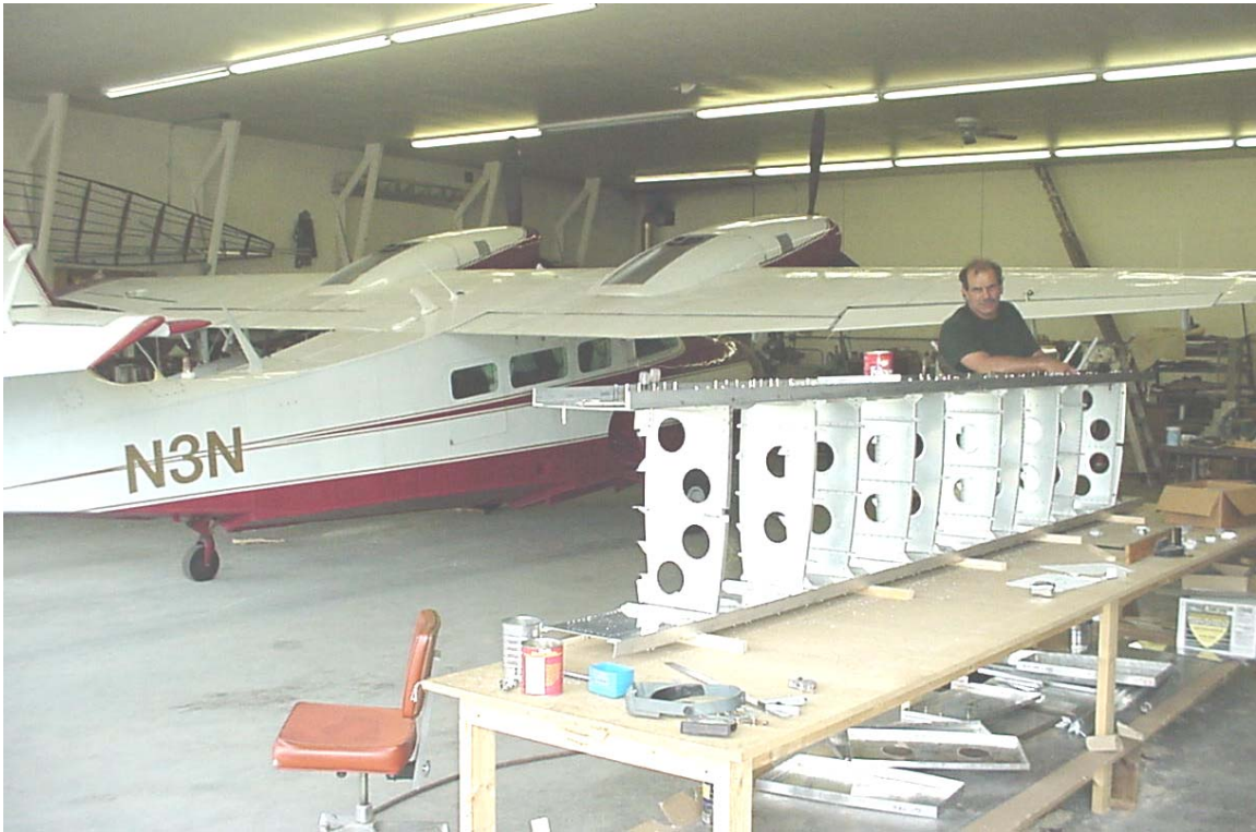
A Unique Hanson industry modernizing 60-Year old Grumman Widgeon amphibians at Cranland Airport - including fabricating major components when needed
