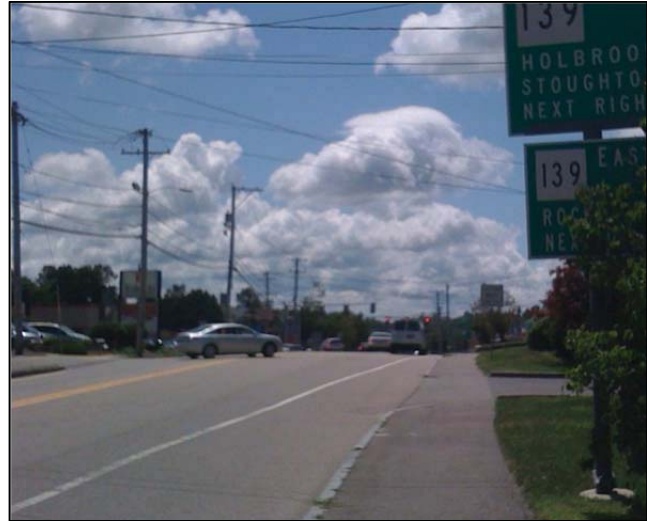
Crest vertical curve limits sight lines of Route 18 southbound approach and lane designations.
