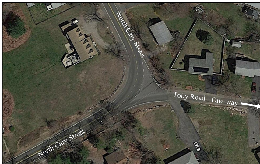
The North Cary Street/Toby Road intersection, North Cary Street curves sharply through the intersection and Toby Road is a one-way street eastbound (away from the intersection).
