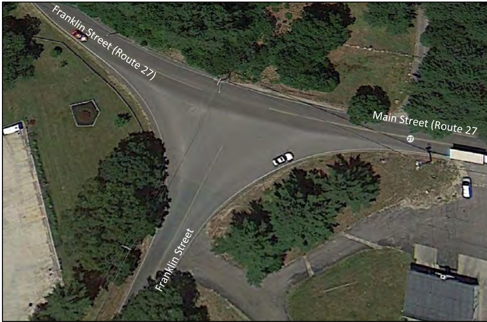
Franklin Street/Main Street (Route 27) intersection showing lack of stop sign and stop line and wide mouth at the Franklin Street approach
