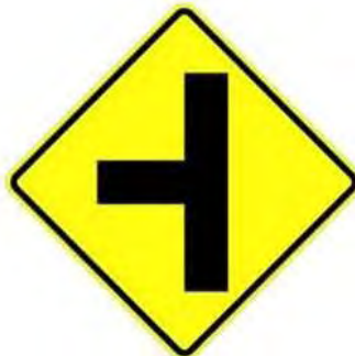
Advanced intersection warning sign W1-10
