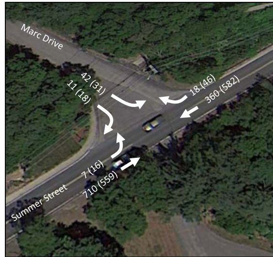
Figure 7 – Turning Movements with Relocated Traffic from Samoset Street/Marc Drive Added to Summer Street/Marc Drive
