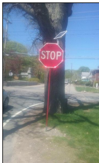
Flashing Stop Sign recently installed by the Town of Stoughton on the westbound approach (there is also one on the eastbound approach)
