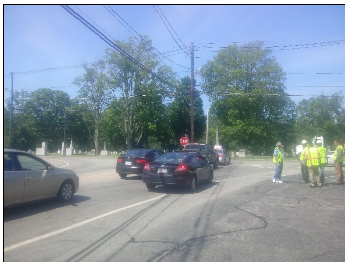
Right turning vehicles on the westbound stop sign controlled Matfield Street approach use the shoulder, which has no curb or sidewalk, as a de-facto right turn lane to bypass traffic waiting to turn left from Matfield Street to North Main Street.
