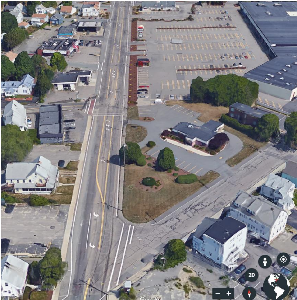
In many locations, the parking areas and asphalt are uninterrupted. Along edges like this, curb cuts should direct vehicle access and sidewalks installed to separate pedestrians from vehicles.
