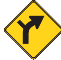
Typical Warning Sign (W1-10) (Source: MUTCD)
