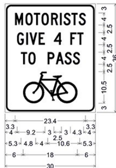
bike passing 35 mph +; 2.0" Radius, 0.5" Border, 0.3" Indent, Black on White; "MOTORISTS", C 2K; "GIVE 4 FT", C 2K; "TO PASS", C 2K; Bicycle;
