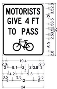
bike passing - under 35 mph; 2.0" Radius, 0.5" Border, 0.3" Indent, Black on White; "MOTORISTS", C 2K 75% spacing; "GIVE 4 FT", C 2K; "TO PASS", C 2K; Bicycle;
