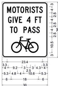
bike passing 35 mph +; 2.0" Radius, 0.5" Border, 0.3" Indent, Black on White; "MOTORISTS", C 2K; "GIVE 4 FT", C 2K; "TO PASS", C 2K; Bicycle;
