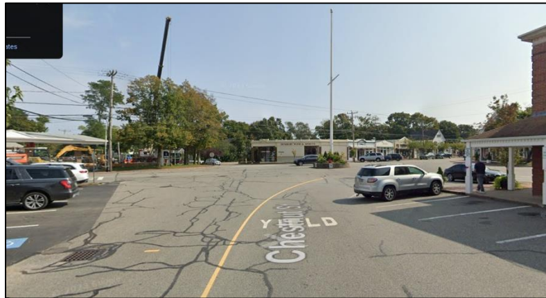
The only control on the Chestnut Street approach is YIELD pavement markings. The proximity of the angled parking results in no available location to post a YIELD or STOP sign.
