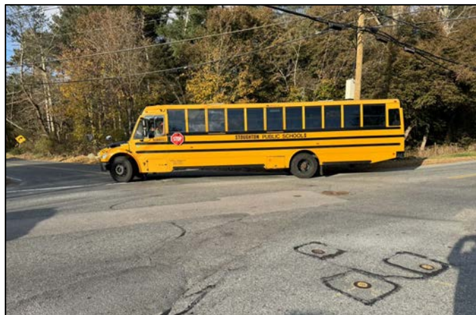
The above photo shows a school bus taking a wide turn due to tight turning radii and utility pole location on the northeast corner of the intersection.
